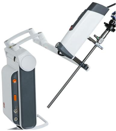
Fig. 3. *AutoLap*, assistant robot that is capable to control the camera during laparoscopic procedures [17].
