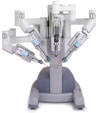
Fig. 2. *da Vinci*, surgery robot used in image-guided laparoscopic procedures. [14]
