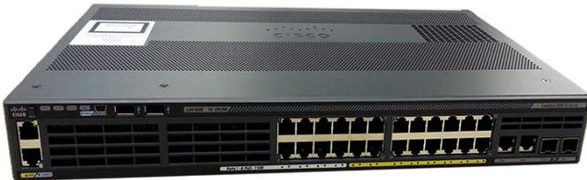
The Cisco Catalyst 2960-X Series adds a new member: the WS-C2960X-24PSQ-L (Cool). This is a 24-port 10M/100M/1000M switch that can power up to 8 ports of PoE (first eight ports only) with ability to deliver a sum total of 110W of PoE power. This switch has four Gigabit Ethernet uplinks: two of them SFP and the other two 10M/100M/1000M copper interfaces enabling choice of fiber or copper connectivity to the aggregation point. This switch ships with the Cisco IOS LAN Base image.
